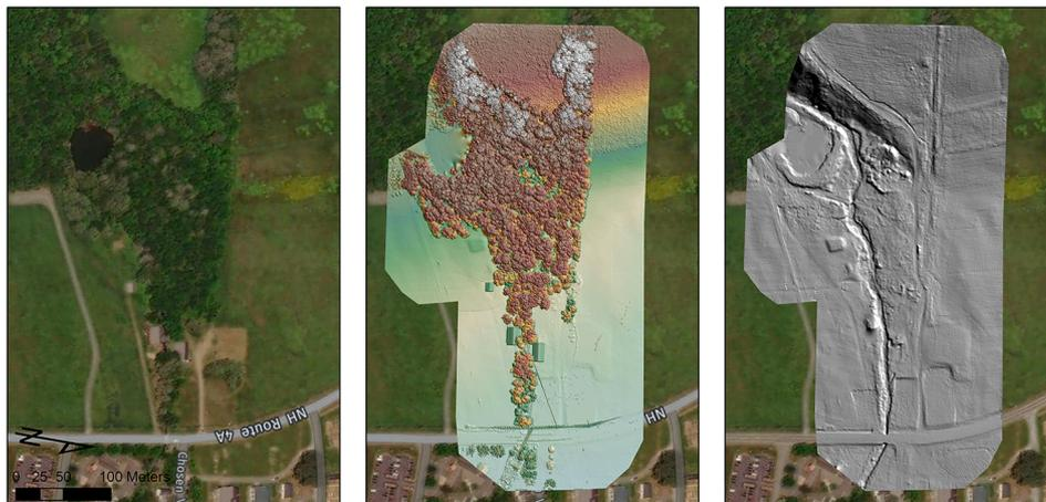
**Fig. 10.** Results of lidar survey at Enfield Shaker Village: A) orthoimage, B) digital surface model illustrating tree canopy as represented by first return lidar, C) bare-earth terrain model hill shade revealing field walls and architectural features below forest cover.
